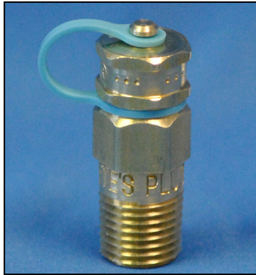
Product: #100 Core: Neoprene Thread: 1/4" NPT Length: 1 1/2"
