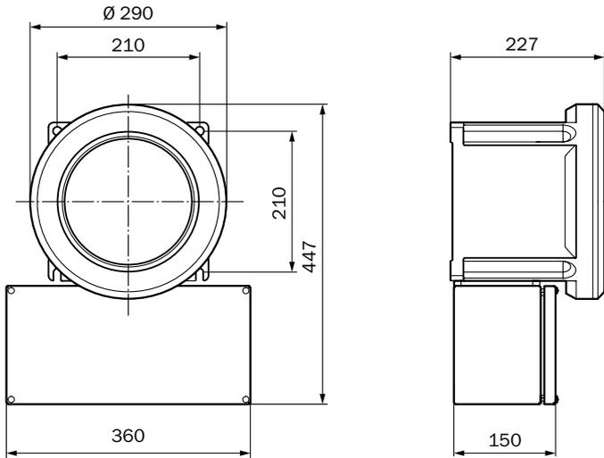
MCUP control unit; wall housing Ex d/Ex e, stainless steel, ATEX zone 1
