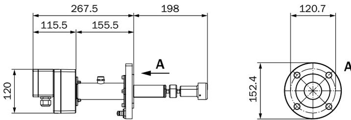
Sender/receiver unit (digital) with electronic unit for ATEX zone 2
