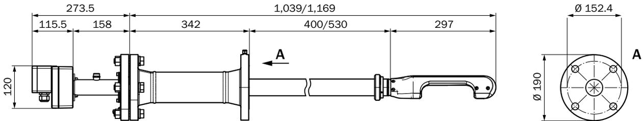
Sender/receiver unit (digital) with electronic unit for ATEX zone 2: Nominal length 400 mm for pipe diameters up to 48"; nominal length 530 mm for pipe diameters > 48" to 72"
