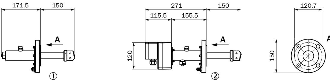
① Sender/receiver unit (analog) for ATEX Ex zone 1, Ex zone 2, and CSA C I I, div 1/div 2
