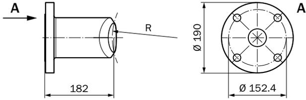
Ball valve, 2" version for standard temperatures
