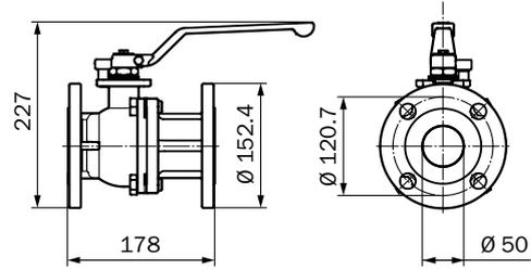
Ball valve, 2" version for high temperatures
