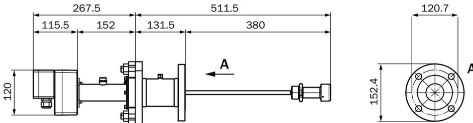
Sender/receiver unit (digital) with electronic unit for ATEX zone 2
