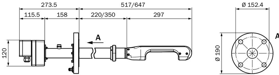
Sender/receiver unit (digital) with electronic unit for ATEX zone 2: Nominal length 220 mm for pipe diameters up to 48"; nominal length 350 mm for pipe diameters > 48" to 72"
